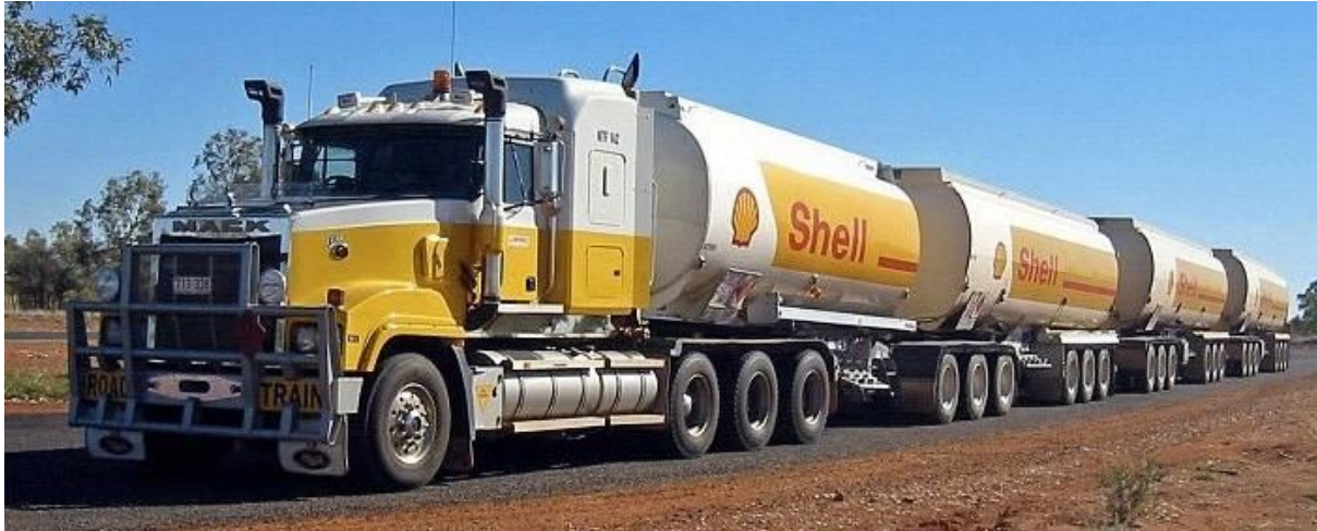
Fuel Road Train (Picture by Thomas Schoch): Fuel Trucks consist of a prime mover followed by one or more trailers, linked using fifth wheel coupling.
